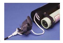
An optional attachment for the LRT is a rope canister that allows items left on the seabed, for example; tools, cables and salvage, to be quickly and easily hauled up.
