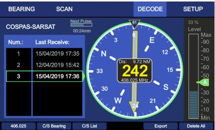
Decode page with direction and distance indication to COSPAS-SARSAT GPS-Position and list of reception history
