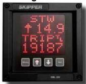
The SKIPPER COMPACT EML 224 is a single or dual axis speed log, working on the electromagnetic principle, providing longitudinal and transversal ship's speed relative to sea water. The COMPACT EML 224 gives accurate navigation parameters, measured as they happen, and presented in a logical, user friendly way.
