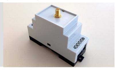
A GPS time-controlled synchronisation pulse harmonised to UTC 00:00:00. With an astronomical clock for day/night light control and external GPS antenna, the GPS can synchronise all Navigation Lights and is suitable for mounting on din rails.
